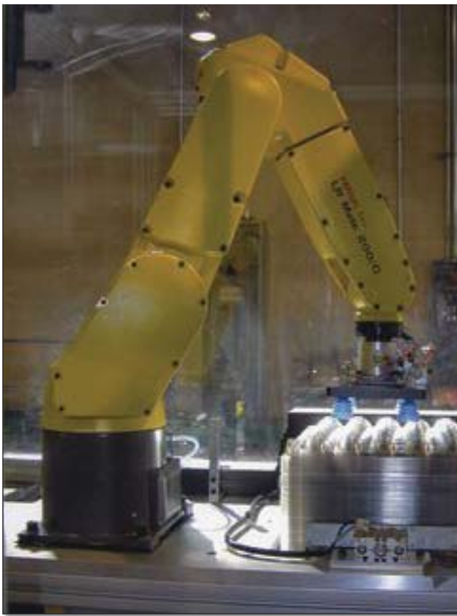
SMR SmartTOPPER™ places pre-formed molded fiber or PET tops on flats or over the top tier of eggs in cases.
