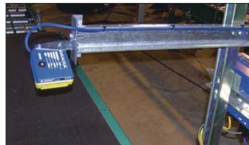
The Smart Motion robotics module verifies bar codes on cases of product on conveyors before presentation to the SmartSTACKER™.
